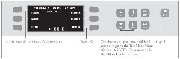
FIGURE 32: Testing the Rack Oscillator
